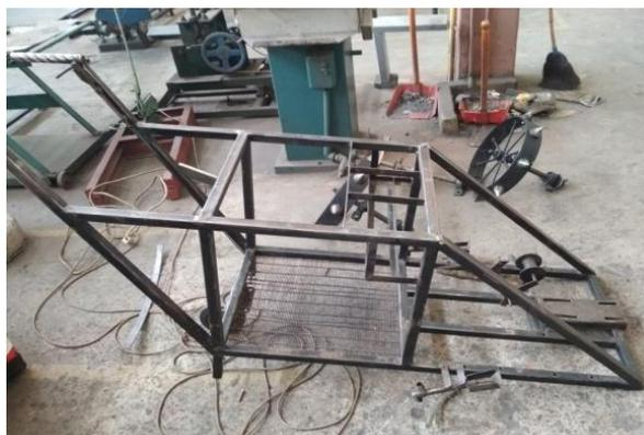
**Gambar 1. Rangka Mesin Penanam Jagung**
