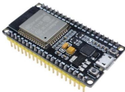
**Gambar 2.** Board Mikrokontroler ESP32
